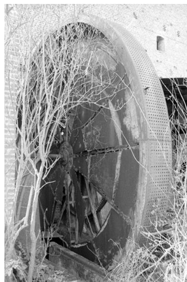
Roue de lavage. Phot. Francis Dubuc IVR22_19908001494Z
